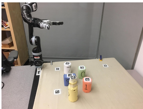
Figure 7.4: Kinova Mico: manipulator arm for Manipulation Subsystem
