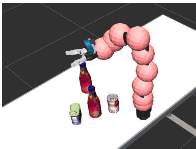
Figure 7.5: CHOMP Planner's approximation of the joints and links
