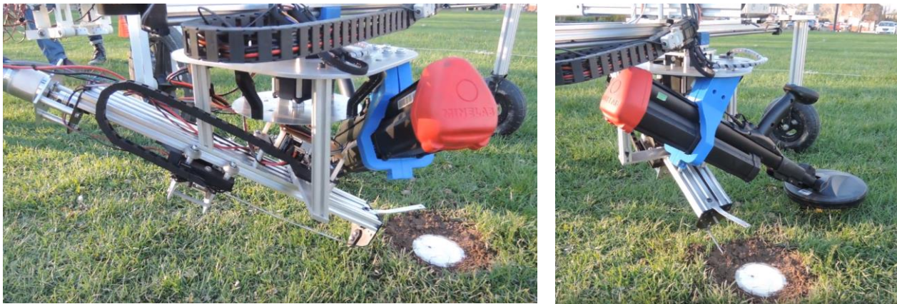
Figure 18: Probe Assembly Mounted on Gantry
