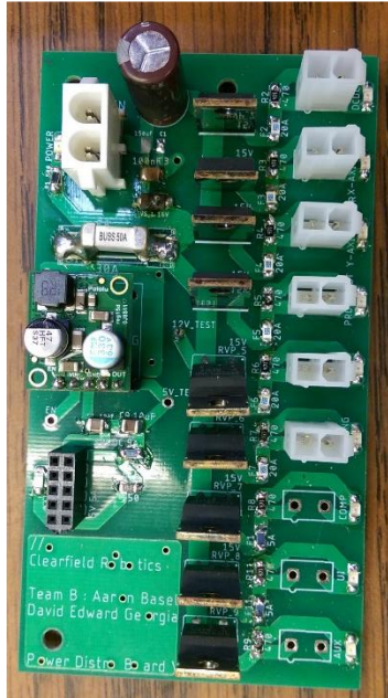
Figure 31: Power Distribution Board
