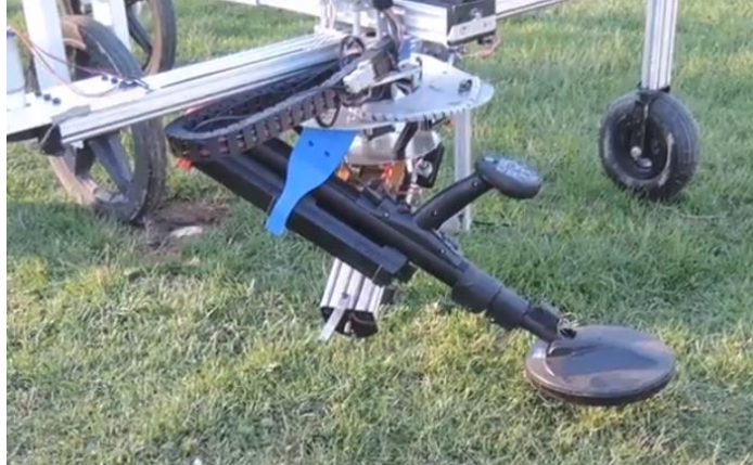
Figure 14: Metal Detector Mounted on Gantry
