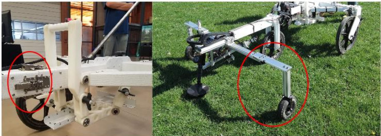
Figure 13: Faulty Clasps (left) and Support Wheels (right)
