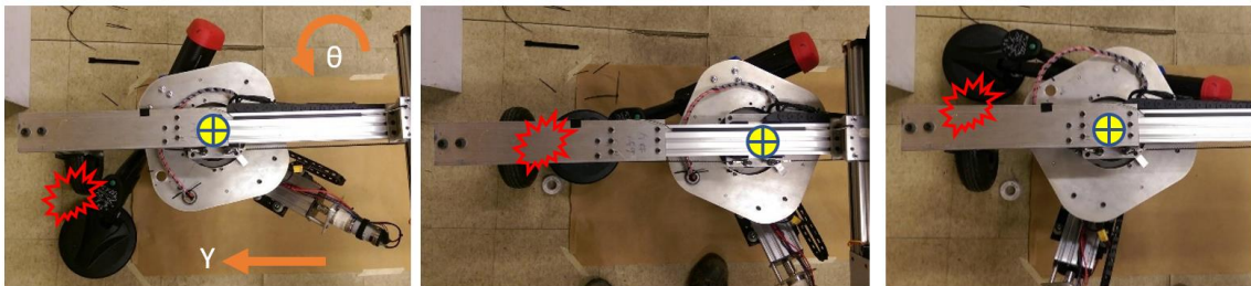
Figure 21: Worst-Case Gantry Transition Condition (Left: Start. Right: End)
