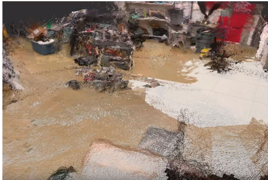
Figure 6: 3D-Map output of RTAB-Map (Real-Time Appearance Based Mapping)
