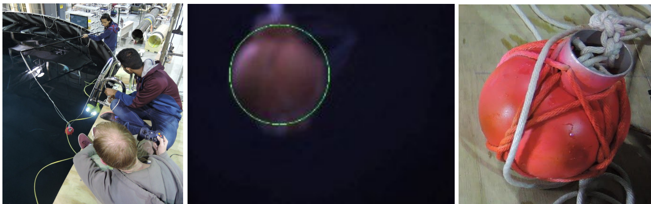
Figure 5: Underwater Ball Detection Set-up, Sample Detection and Target
