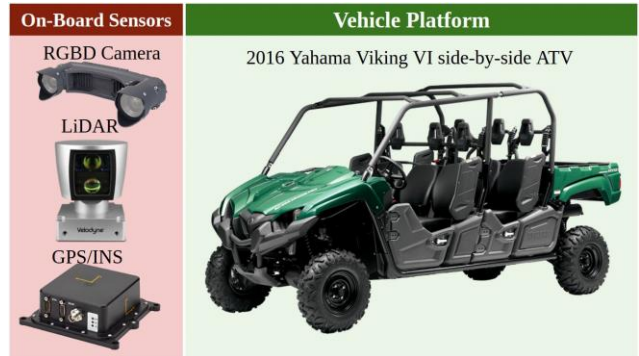
Figure 1. The testing vehicle platform and the on-board sensor.
