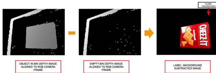
Figure 5: The Automatic Labeling Mechanism
