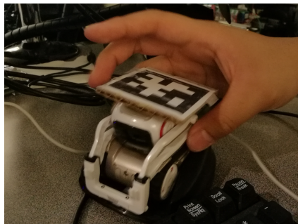
Figure 4: The Anki Cozmo has an APRILTag placed atop it to allow for smooth tracking. It was programmed using the SDK via an iOS phone.
