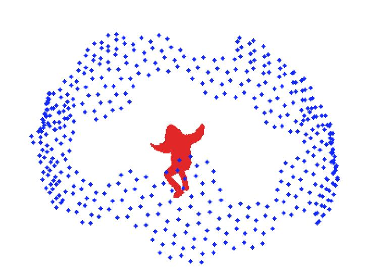
The 3D reconstruction of the subject is done using the Visual Hull Algorithm and images from all 480 cameras.
