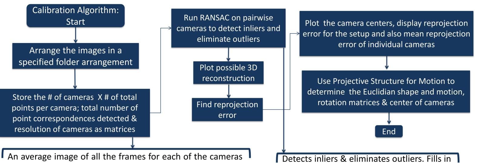
is computed, which contains all detected LED points. An image of standards deviation is computed from the average image by estimating the position of the 3D points.
